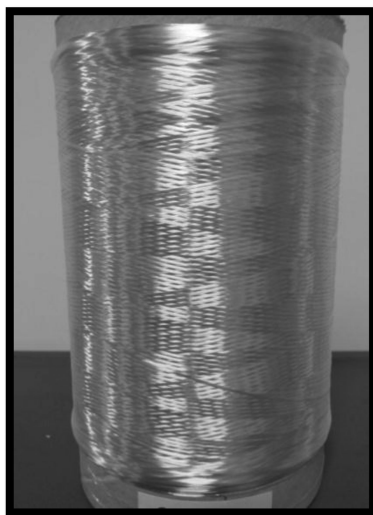
Figure 6. An example of multi-filament, continuous PAN precursor tow, dry-jet spun at the University of Kentucky Center for Applied Energy Research.
