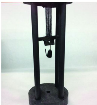
Figure 8. Fiber tow suspended on a customized graphite rack and tungsten weight loaded at the bottom.
