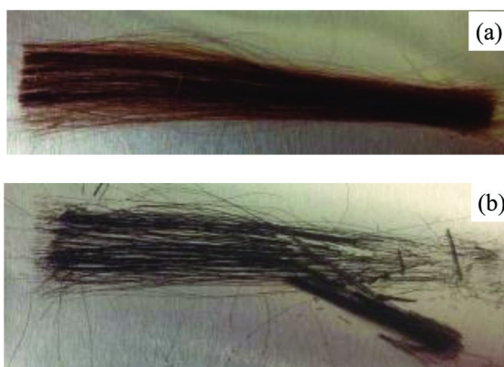
Figure 2. (a) as-spun Ace-SKL fibers; (b) tacky Ace-SKL fibers after thermal stabilization.
